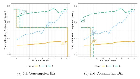
Figure 3: Optimal System Sizes for Two Example Consumption Levels. Figure shows the marginal per-kWh price of solar generation for the subset of homes from Figure 2b along with the marginal grid price (dashed line) for consumption. Optimal installation sizes are indicated with "\*" for each house.
