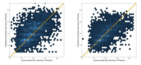
Figure C.2: Density plot of Google Sunroof-method predicted (y-axis) and actual (x-axis) installed system capacity for (left) purchased systems inclusive of rebound and (right) leased systems. The diagonal represents correct predictions of the optimal installation size.
