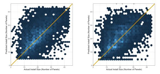
Figure C.1: Density plot of Google Sunroof-method predicted (y-axis) and actual (x-axis) installed system capacity sized using (left) actual consumption and (right) using assigned closest consumption bin, both inclusive of rebound. The diagonal represents correct predictions of the optimal installation size.
