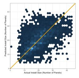
Figure B.2: **Sizing model accuracy**. Density plot of Google Sunroof-method predicted (y-axis) and actual (x-axis) installed system capacity for (left) purchased systems and (right) leased systems. The diagonal represents correct predictions of the optimal installation size.
